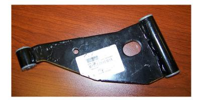
To install the new bushings clean the bore and clean off any burrs that may exist.
