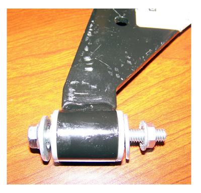
Next install the sleeve. Again lubricate the sleeve and bushing. Install a 5/16" rod (all thread) into the sleeve with washers on either end. Tighten the nuts until the sleeve fully draws into the bushings. Then remove the rod and tap sleeve with a hammer to center it.
